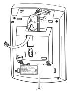
5. Plug the short modular cord's other end into the wall plate jack, align the base's keyhole slots with the wall plate studs, and slide the base downward to secure it.
